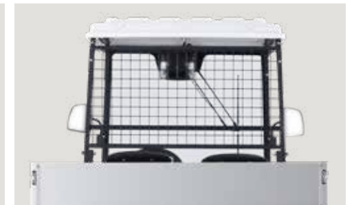
Driver Protection Steel Plate
