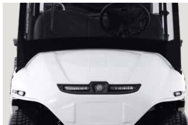
Standard LED Lighting System
